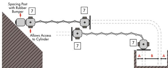
Pocket doors (supplied by others) should be hinged to interior for curtains with self-locking travelling end post.
