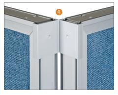
Each panel includes removable gray plastic caps to enable easy connector fitting. Align panels, slide connector into slots, and gently tap into place with a rubber mallet.
