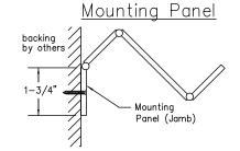
Direction of mounting panel (jamb) varies based on door construction. Consult factory for specific information.
